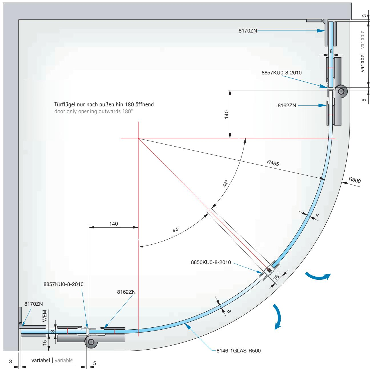
WEM = Wanneneintrückmaß (15mm) | distance between the outer edge of the side part and the outer edge of the shower basin (15 mm)
