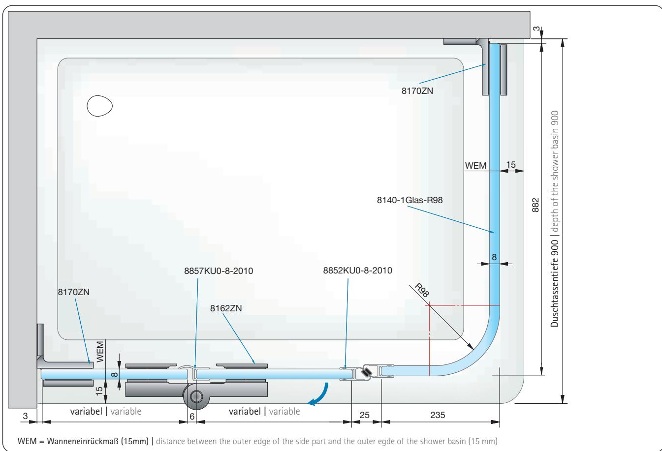
WEM = Wanneneinrückmaß (15mm) | distance between the outer edge of the side part and the outer edge of the shower basin (15 mm)
